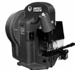
AMP-O-LECTRIC Bench Machine with Special Applicator
